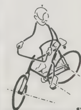
822. WHEELS ON DIFFERENT AXES. The short-axis rule applies, no matter which way the axle slants.
